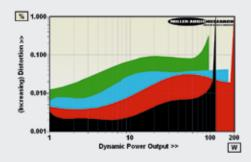
ABOVE: Dynamic power output versus distortion into 80hm (black trace), 40hm (red), 20hm (blue) and 10hm (green) speaker loads. Max. current is 9.8A
