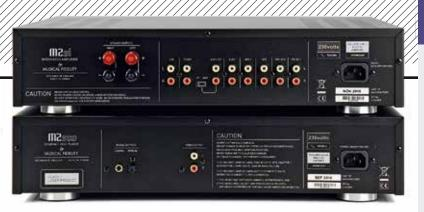
**ABOVE:** Five line inputs, a tape loop and pre outputs join single sets of (switched) 4mm speaker cable terminals on the amplifier [top]. The CD player [bottom] has no digital inputs – just analogue output on RCAs and S/PDIF out on coax and optical
