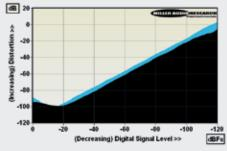
ABOVE: THD versus 16-bit CD digital signal level over a 120dB range at 1kHz (black) and 20kHz (blue)
